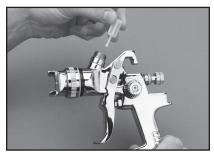
Figure 3. Installing filter.
